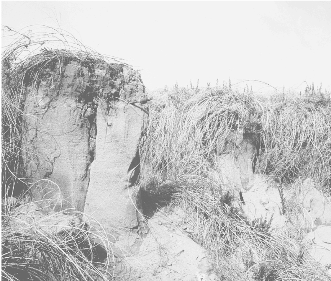
Figure 3.9 Profile of a Psamment formed on sandy alluvium in Virginia. Note the accumulation of organic matter in the A horizon but no other evidence of profile development. The A horizon is 30 cm thick. (Photo courtesy of R. Weil)
